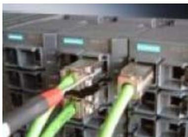
Figure 4-7 Releasing the RJ-45 Plug with a screwdriver
