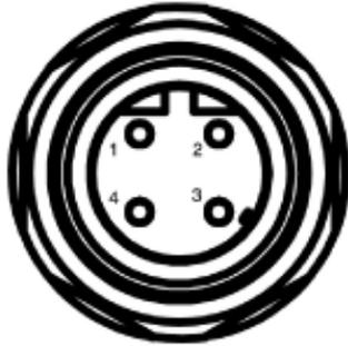
Figure 3-4 SCALANCE 208PRO Ethernet socket M12
