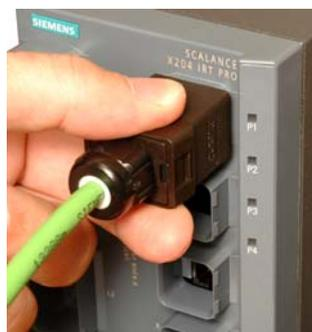
Figure 4-10 Removing IE RJ 45 Plug Pro or IE SC RJ Plug Pro
