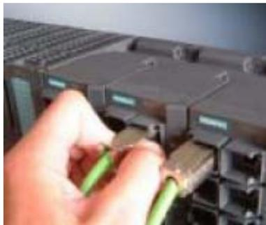
Figure 4-6 Releasing the RJ-45 Plug
