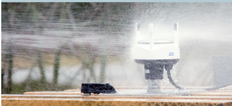
Water protection test
